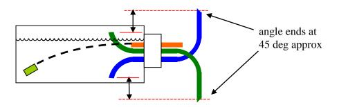
The significant points are that the layout is symmetrical whether it's upright or inverted and that the external ends of the pipes finish above or below the max and min fuel levels, as shown by ------, in order to prevent fuel outflow whilst stationary.
